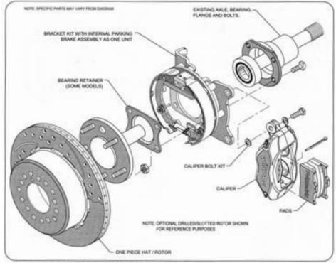
Typical Dynalite Pro Series Rear Parking Brake Kit, Major Components Identified (Vented Version Shown)
