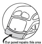
complete bottom flange. Die stamped of 18-gauge steel.
